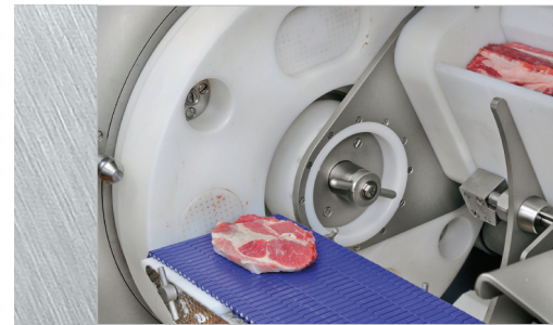
The rotating chamber system allows the continuous infeed of the raw material.
