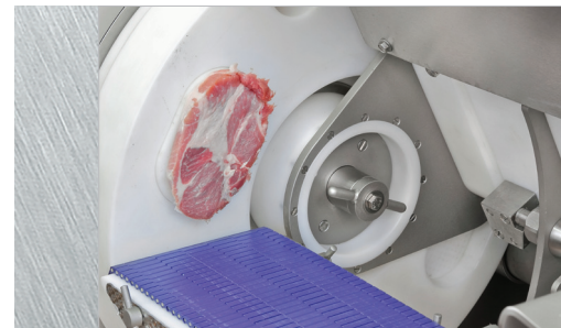
The rotating chamber system allows the continuous infeed of the raw material.
