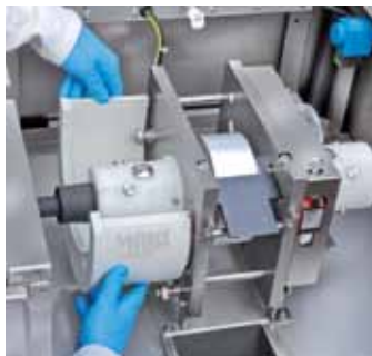
Removal of the water tank for cleaning purposes
